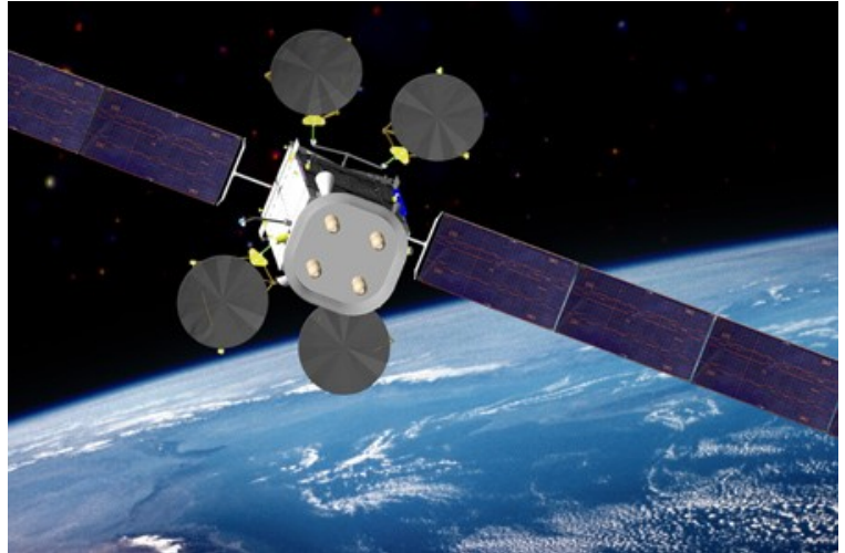
Boeing introduced the 702MP spacecraft in 2009 to meet the needs of customers seeking satellites in the middle-level power ranges. Its flexible design supports payloads that range in power from six to 12 kilowatts. (image of Intelsat’s IS-22 satellite courtesy of Boeing)
