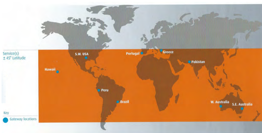
O3b’s service coverage area at 45° latitude north and south of the equator. Connectivity to the fiber infrastructure can be made through Gateway locations at key cities worldwide. (image courtesy of O3b Networks)
