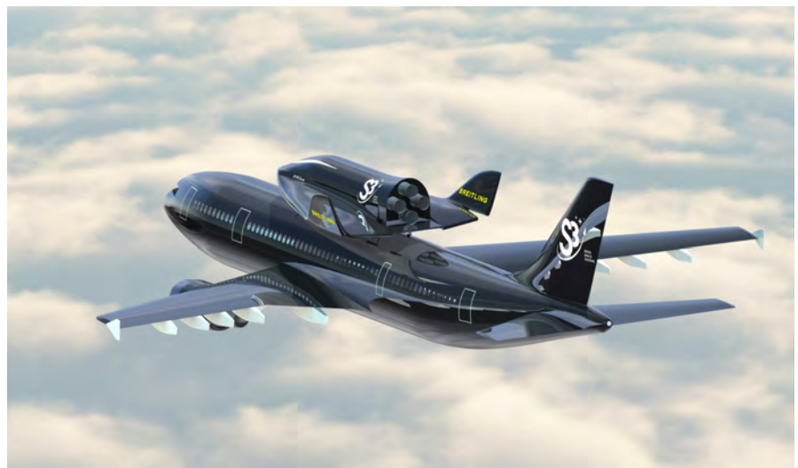
Artist’s rendering of S3’s Suborbital Aircraft Reusable shuttle (SOAR). It features a three-stage configuration consisting of an Airbus A300 jumbo jet using standard fuels, a suborbital spacecraft that piggybacks on the Airbus, and a disposable third stage shuttle that is used to deploy satellites. (image courtesy of S3)
